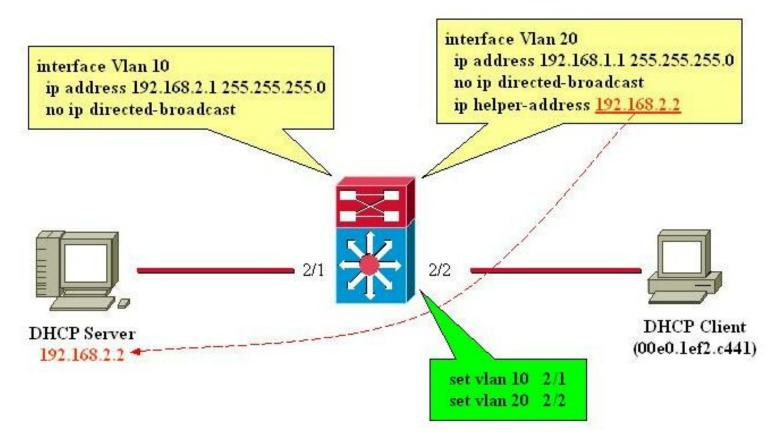
As configured in the diagram above, interface VLAN20 will forward the client's broadcasted DHCPDISCOVER to 192.168.2.2 via interface VLAN10. The DHCP server will fulfill the request via unicast. No further configuration to the router is necessary in this example. The switch ports will need to be configured as host ports and have Spanning-Tree Protocol (STP) portfast enabled, and trunking and channeling disabled.
