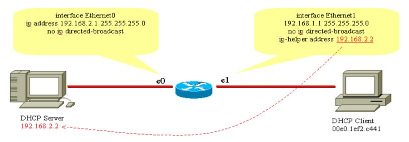
To forward the BootP/DHCP request from the client to the DHCP server, the **ip helper-address interface** command is used. The IP helper-address can be configured to forward any UDP broadcast based on UDP port number. By default, the IP helper-address will forward the following UDP broadcasts:
