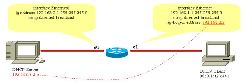
Scenario 1: Cisco Router Routing between DHCP Client and Server's Networks
